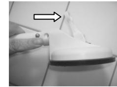
For the exchange of the suction head press the interlock at the side and draw off the suction head in direction of the arrow. Push the new suction head until it lock clearly.
