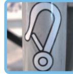
If the wheelchair must be lifted with an articulated crane, to hurdle obstacles, you must not use spots other than the 4 marked with a hook sticker as shown here.
