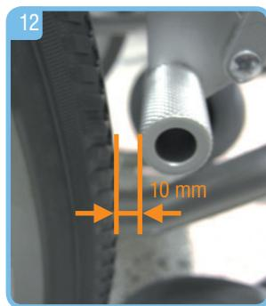
**⚠ Make sure, that both sides are adjusted correctly and on the same height.**
