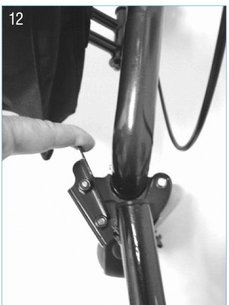
13 in such a way that all 3 bolts have engaged, then the footrests are firmly arrested at the Rollator (picture 14).
